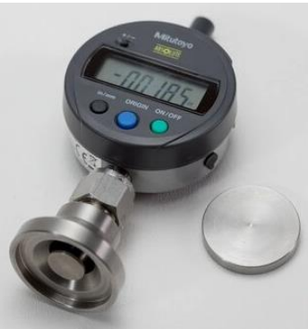
Figure 3. Minor Stem Height Measuring and Zero Calibration Block example.
