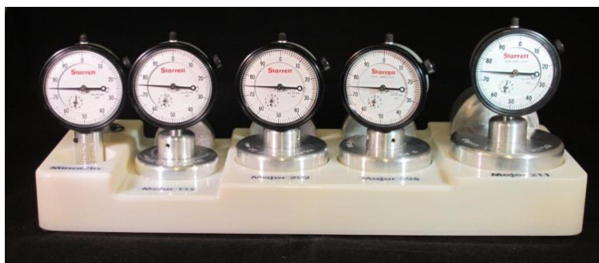
Figure 1: Starrett Stem Height Gauges
