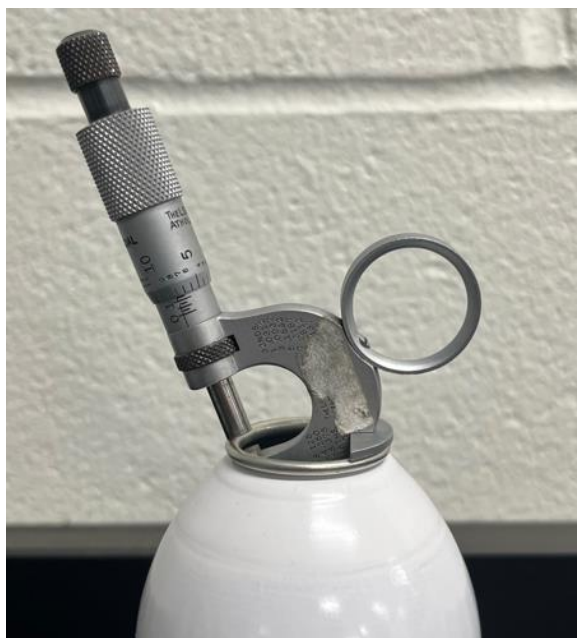
Figure 1. Curl Thickness Measurement Example
