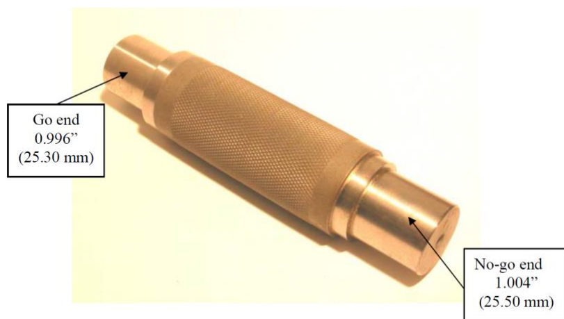
Figure 1. Go/No-Go Bar Gauge
