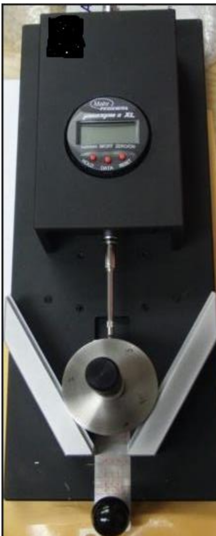
Figure 2. Example of a Measuring Fixture with a Diameter Calibration Gauge Block.
