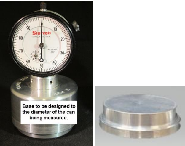
Figure 3. Minor Stem Height Measuring and Zero Calibration Block example.
